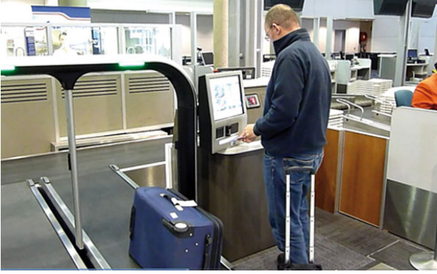
Fig. 8. Self baggage drop system in Brisbane airport: baggage is collected and carried to determined destinations using several conveyor belts.
